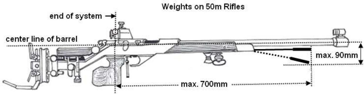
Weights on the fore-end of the rifle may extend no lower than 90mm below the center line of the barrel and not further forward than 700mm from the back (rear) end of the system
